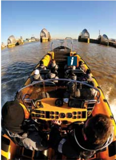
chase across open water at 50 knots they are going to need a more robust system. As a simple rule, a suspension seat that ‘bottoms out’ is potentially more damaging than having a non-suspension seat.
